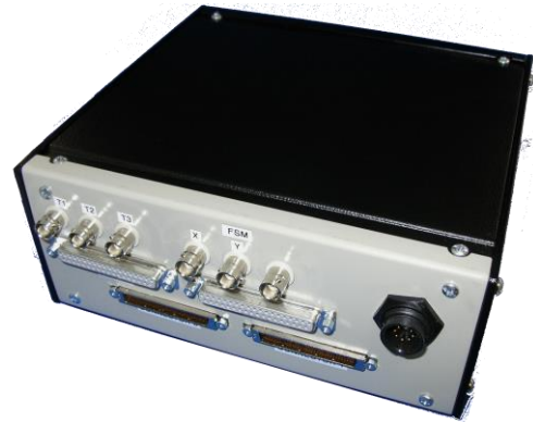
Figure 2 – High-Power SPI Drive Electronics with Optional Analog Output and Triggering BNC Connections
