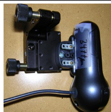
Figure 7.1.1 - Mounting the AOS Hartmann Sensor to a Thorlabs KM100P kinematic prism mount
