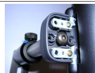
Figure 7.1.2 - Mounting of the USB Webcam Hartmann sensor to a standard 1/2" post.
