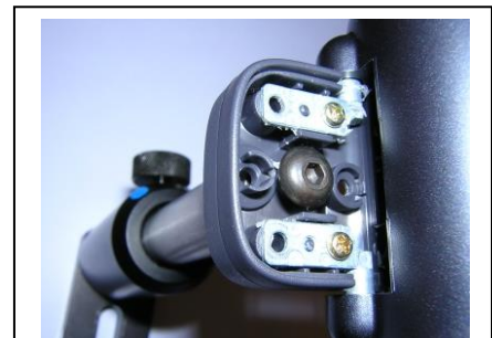
Figure 7.1.2 - Mounting of the USB Webcam Hartmann sensor to a standard 1/2" post.
