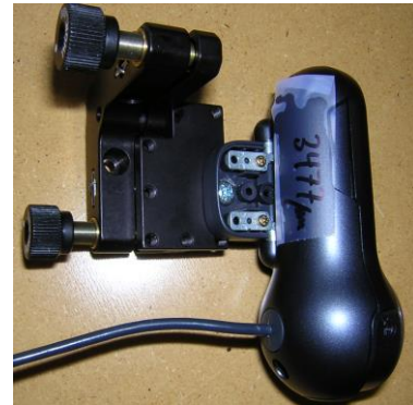
Figure 7.1.1 - Mounting the AOS Hartmann Sensor to a ThorLabs KM100P kinematic prisim mount
